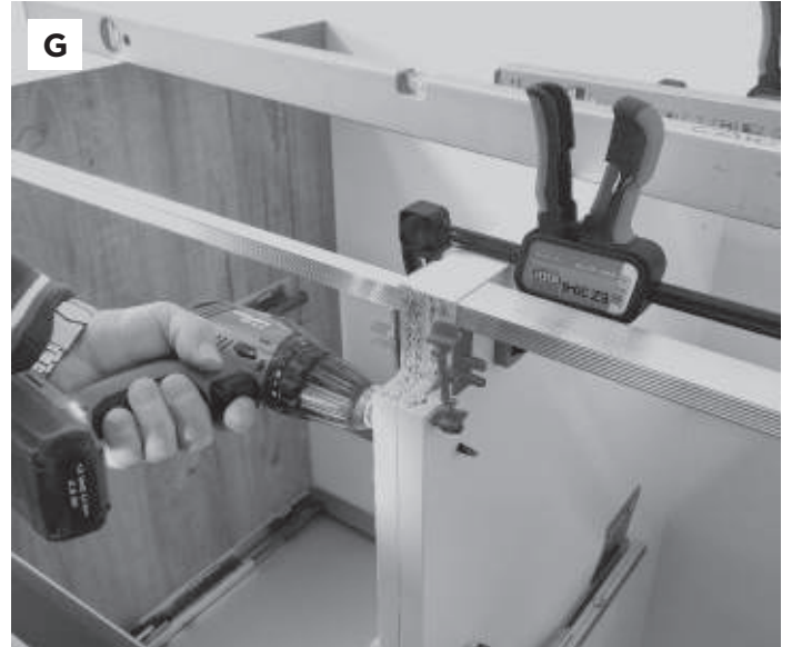
Insert the couplings in the drill holes provided.
